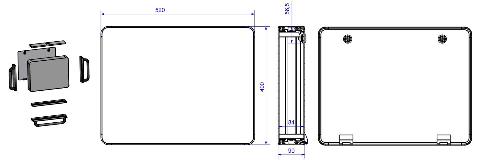
useable front-plate area = 350x470mm area reduction generated by lock and hinge combination
