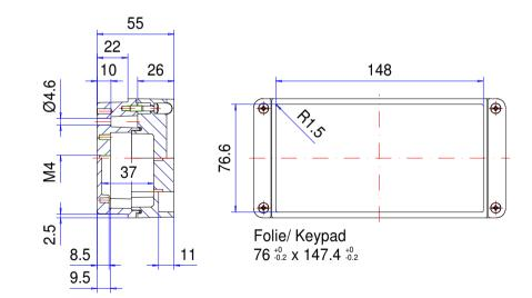
\* Please note: Mould slope for casting ejection, dimensions in the amount of the bottom!
