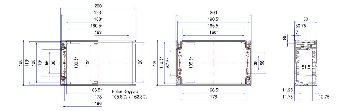
\* Please note: Mould slope for casting ejection, dimensions in the amount of the bottom!
