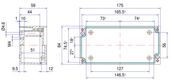
\* Please note: Mould slope for casting ejection, dimensions in the amount of the bottom!
