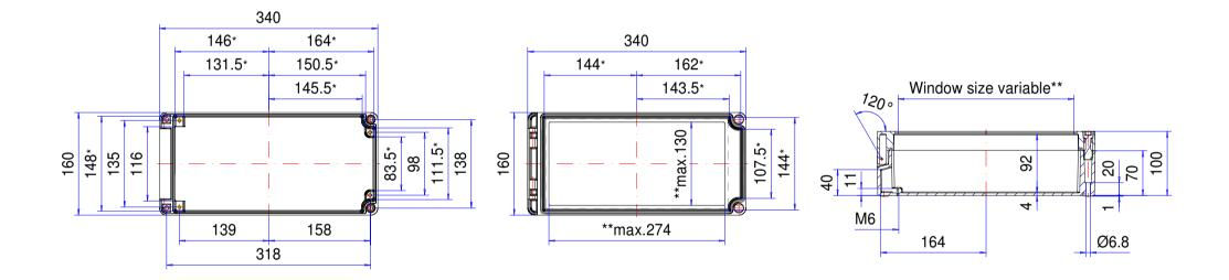
\* Please note: Mould slope for casting ejection, dimensions in the amount of the bottom!
